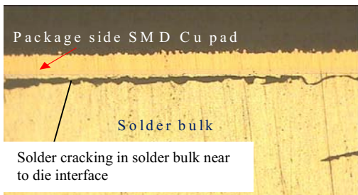
Figure 14: Optical micrograph showing solder crack.
