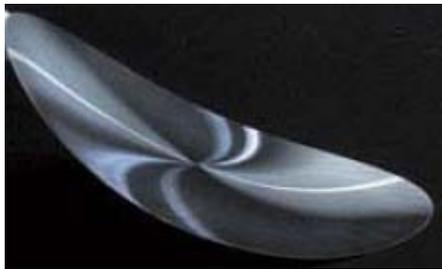
Figure 9: Wafer thinning mark on backside of wafer (Courtesy of Disco Corporation)
