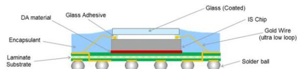
**Figure 5 – Schematic of the iBGA2 package structure, with cover glass extending over the wire bonds**
