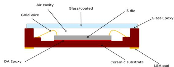
**Figure 2 – Schematic of a CLCC ceramic image sensor package structure**
