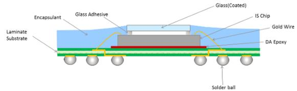
**Figure 3 – Schematic of the iBGA package structure, with cover glass inboard of the wire bonds**
