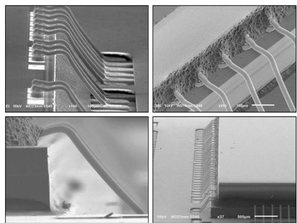
**Figure 6 – SEM images showing ultra-low wire loops (top left), wires embedded in glass attach adhesive (top right & bottom left), and cover glass attached over wire bonds (bottom right), in an iBGA 2 package**
