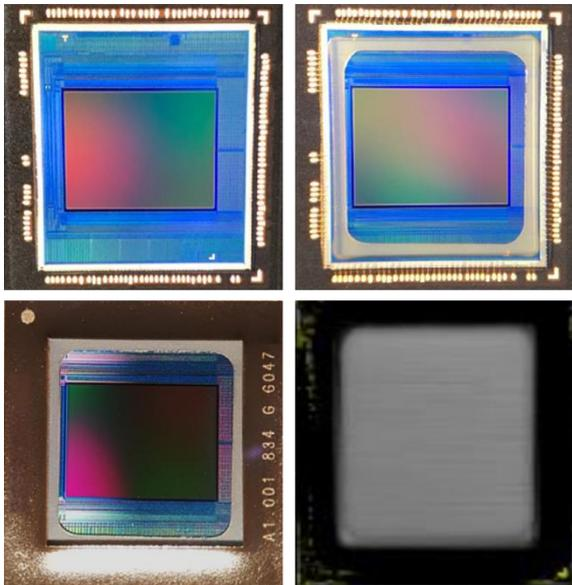
Figure 8 – iBGA package top view after: IS die attach (top left); wire bonding & glass attach (top right); encapsulation, laser marking, ball attach & singulation (bottom left); and after SAM delamination check post reliability stress testing (1000TC / 1000hr THB / 1000hr HTSL), with no delamination observed (bottom right).
