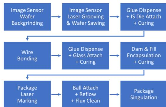
**Figure 4 – iBGA package assembly process flow**
