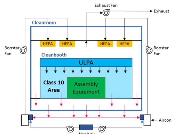
**Figure 1 – Schematic of Class 10 cleanroom booth setup used for CIS package assembly**
