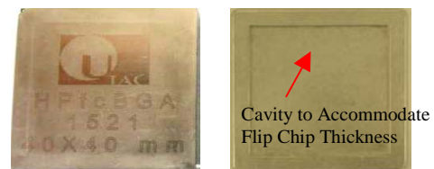
Fig 2. 40x40mm Copper Heat Spreader of HP-fcBGA.
