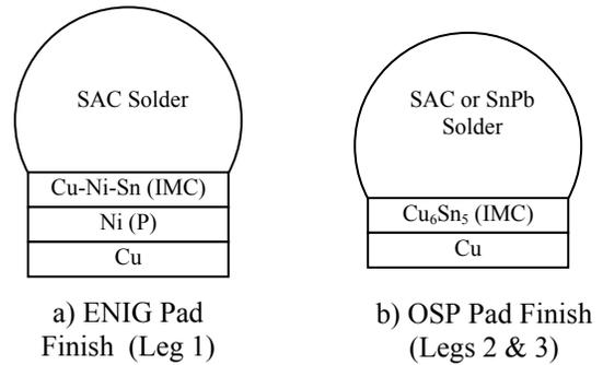
Fig 10. Intermetallic Layers Formation for Legs 1-3.
