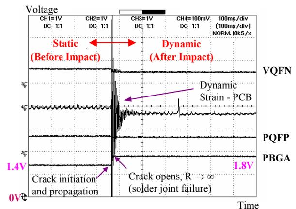
Fig 4. Dynamic Responses for Leg 1 (Pb-free on ENIG) Test Board at 1<sup>st</sup> Drop.
