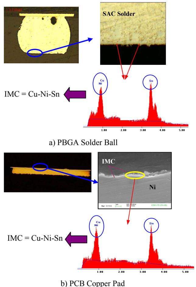
Fig 11. Interfaces of a PBGA Detachment Joint (Leg 1).
