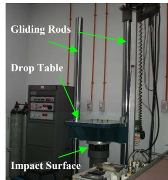
Fig 1. Lansmont Model 65/81 Drop Impact Tester.
