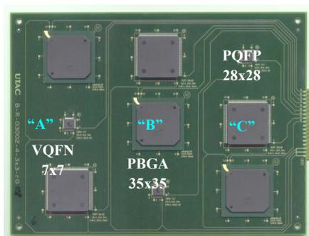
Fig 2. 150x200mm PCB with Drop Test IC Packages.
