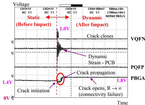
Fig 5. Dynamic Responses for Leg 2 (Pb-free on OSP) Test Board at 15<sup>th</sup> Drop.
