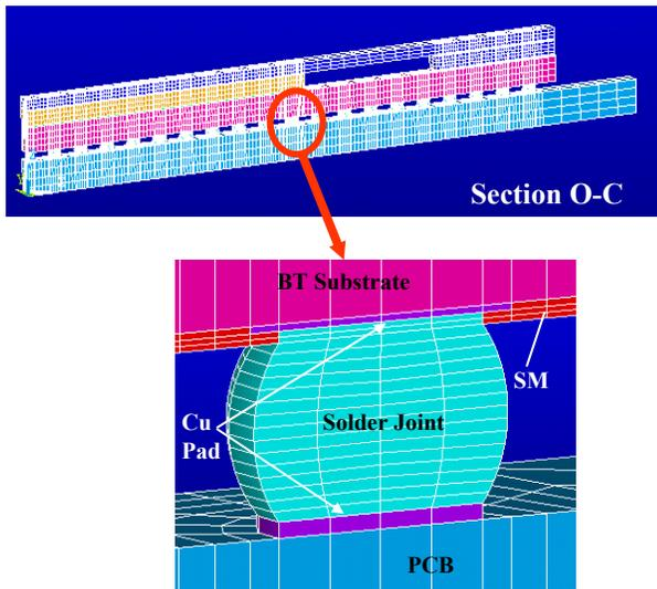
Fig 3 (cont'd). Package Cut-out for the 3D Quarter and 3D Slice Models.
