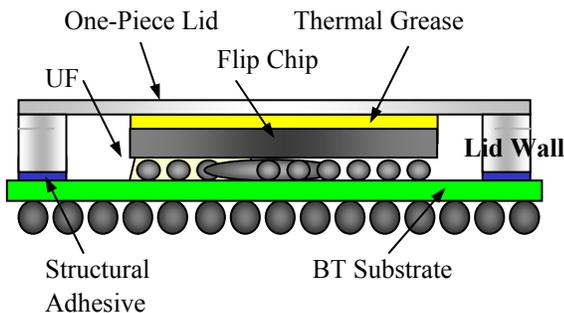
Fig 2. Schematic Diagram of a One Lid HP-fcBGA Package.
