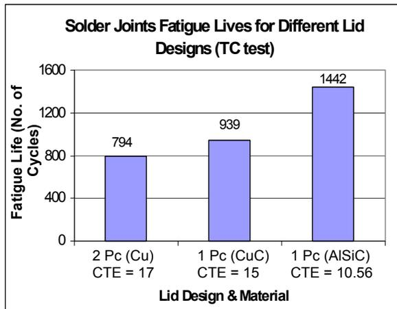
Fig 10. Solder Joint Fatigue Life for Lid Type and Material Comparison.
