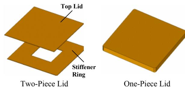
Fig 1. Designs of Two-Piece and One-Piece Lids.
