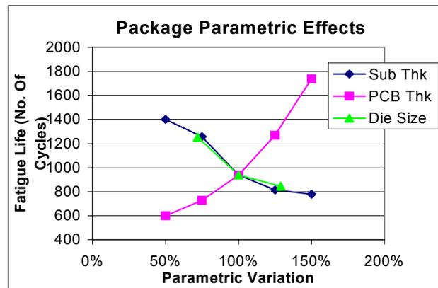
Fig 11. Package Parametric Effect on Solder Joint Reliability.
