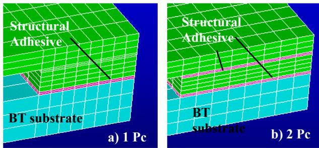
Fig 4. One Pc versus Two Pc Heat Spreader Build Up.
