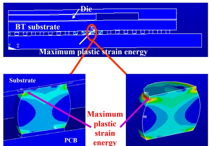
Fig 9. Maximum Strain Energy in the Solder Joint.
