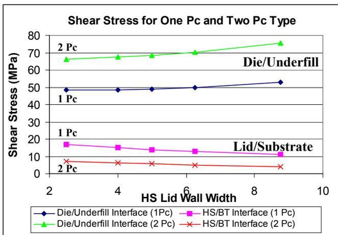
Fig 8. Shear Stresses for Different Lid Types.
