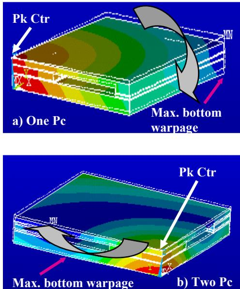
Fig 6. Package Warpage (from 150°C to 25°C).
