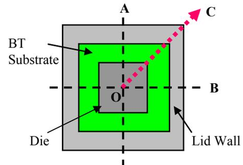
Fig 3. Package Cut-out for the 3D Quarter and 3D Slice Models.
