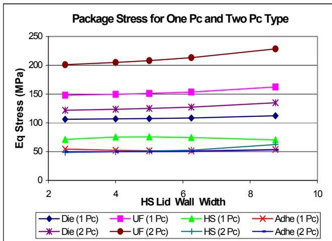
Fig 7. Package Stresses for Different Lid Types.
