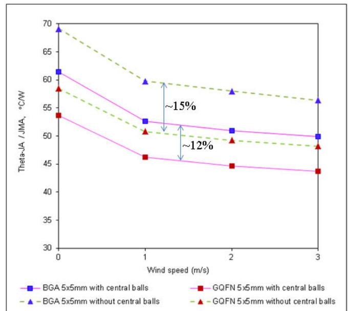
Figure 9: Thermal resistance Junction to Ambient/Moving Air versus Wind speed.
