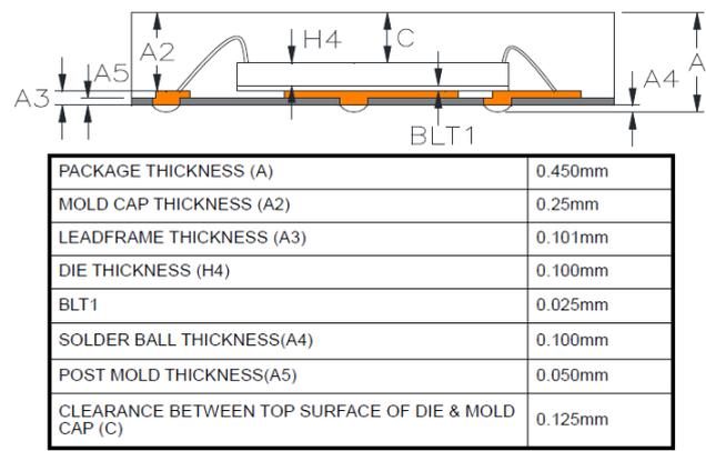
Figure 6: xGQFN package cross section /stackup
