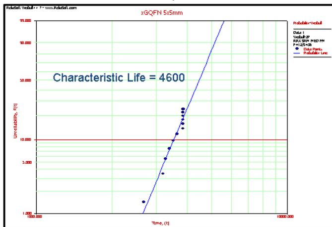
Figure 20: Weibull plot for TCoB characteristic life.
