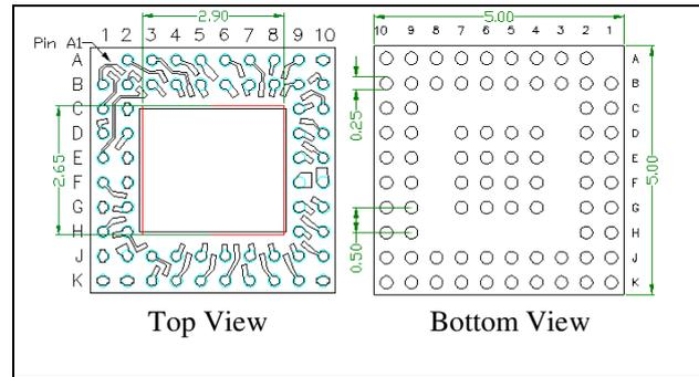
Figure 5: xGQFN 5x5mm 79L Top and Bottom View
