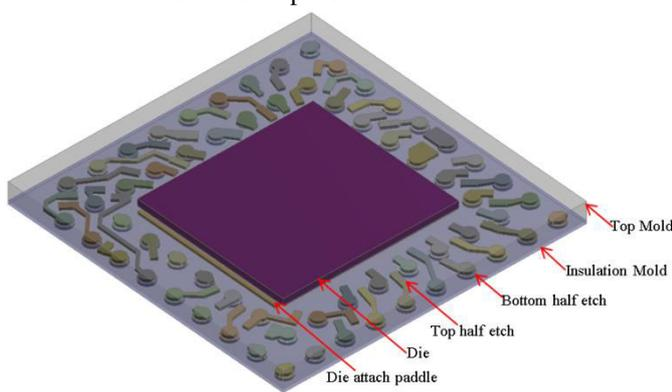
Figure 4: Package structure used in this study (xGQFN)
