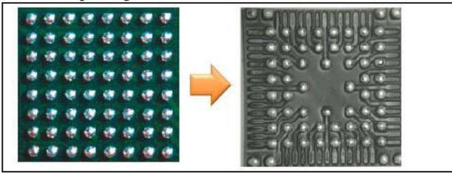
Figure 3: Conversion of laminate package to GQFN
