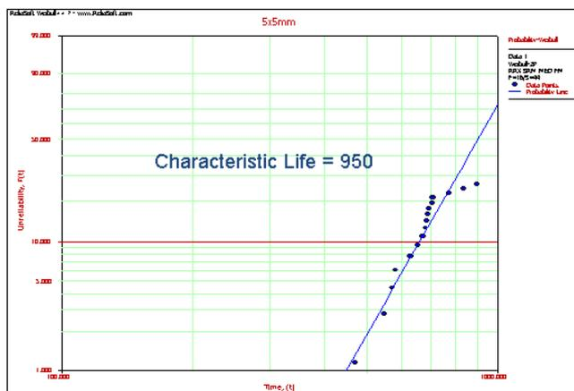
Figure 15: Weibull plot for drop test characteristic life.
