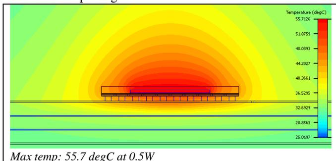
Figure 7: Temperature distribution around the package with 4x4 array of central balls. (BGA 5x5mm at Still Air Test on 2S2P PCB)
