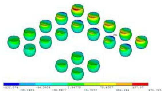
Figure 18: Solder joint stress density
