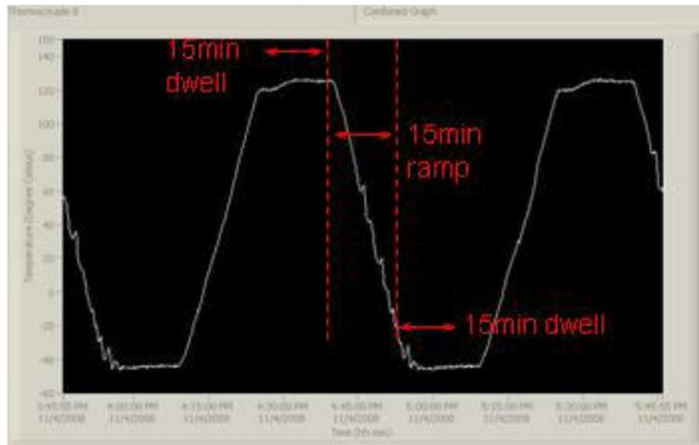
Figure 19: TCoB temperature cycle profile
