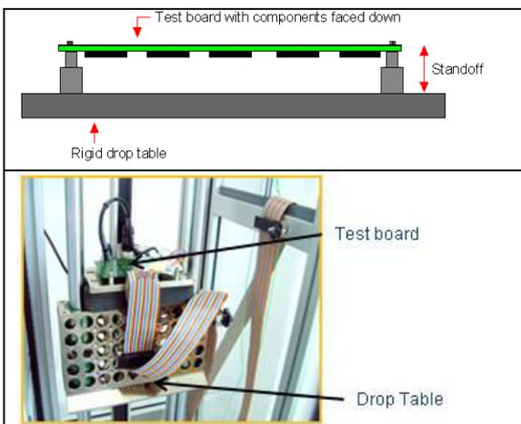
Figure 14: Test board mount and drop test setup
