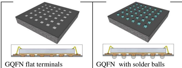
Figure 1: Package structure and cross section of GQFN
