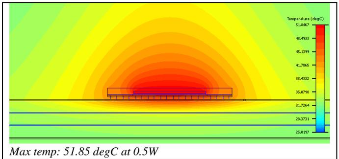
Figure 8: Temperature distribution around the package with 4x4 array of central balls. (GQFN 5x5mm at Still Air Test on 2S2P PCB)
