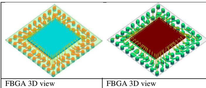
Figure 10: 3D view of both packages with wirebond
