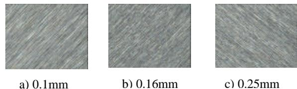
Fig 7. Microscopic Images of Die Backside Surfaces for New Test Wafers.
