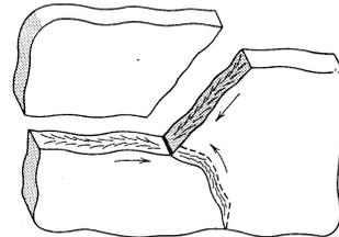
Fig 2. Multiple Chevron Patterns Emanating From Crack Origin [6].
