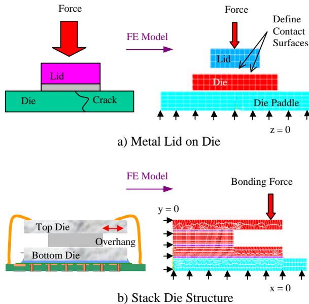
Fig 15. Case Studies for Finite Element Simulations.
