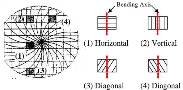
Fig 4. Backgrinding Pattern Corresponding to Different Positions of the Wafer and Bending Axis.
