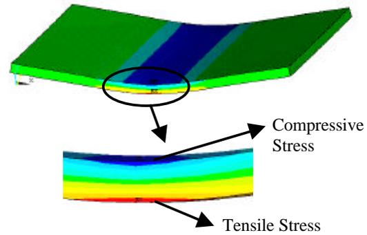
Fig 13. Contour Plots of Silicon Die after Loading.
