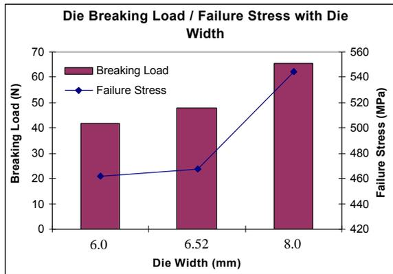
Fig 8. Die Breaking Load and Failure Stress for Different Die Sizes.
