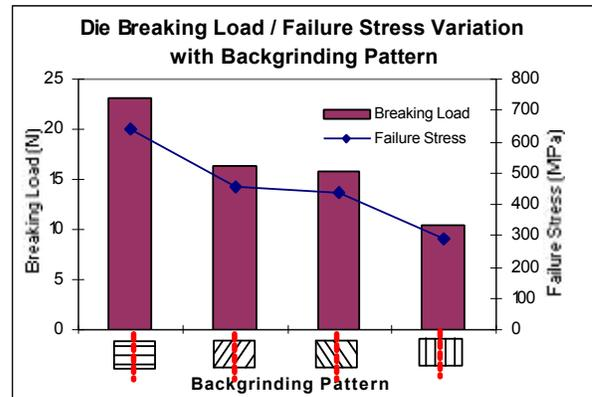
Fig 10. Die Breaking Load and Failure Stress for Different Backgrinding Patterns.
