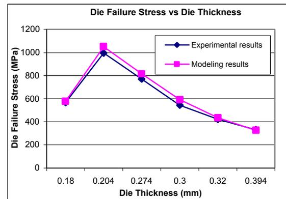
Fig 14. Correlation of Simulation and Experimental Results on Die Bending Test.
