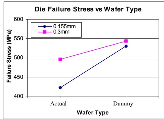
Fig 9. Comparison in Die Strength of Different Wafer Types.
