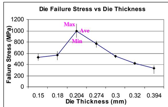
Fig 6. Die Failure Stress for Different Die Thickness.
