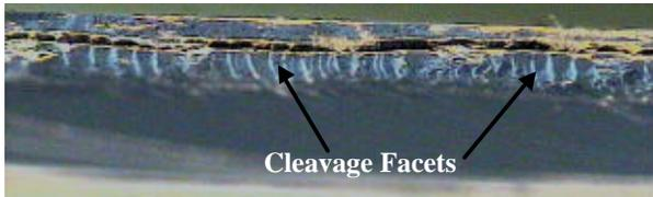
Fig 11. Surface of a Fracture Silicon Die Showing Cleavage Facets.
