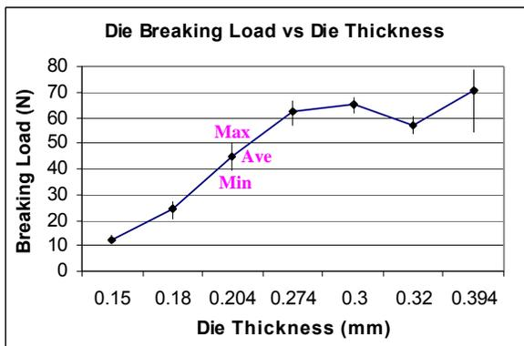
Fig 5. Die Breaking Load for Different Die Thickness.
