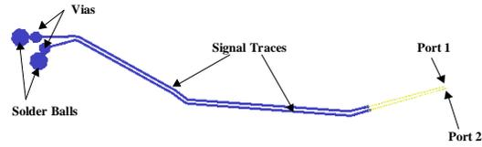
b. Top view with ports assigned at the bond wire ball side
