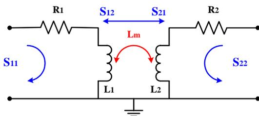
Fig. 4: Two-port RL equivalent circuit of two neighboring signal path
