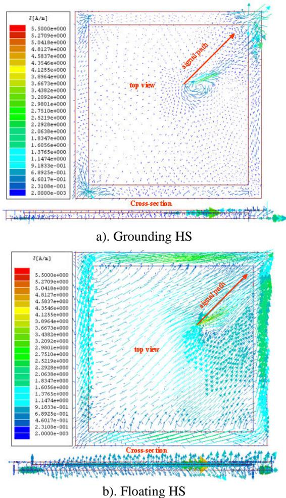
Fig. 10: Surface current plot of a).grounding and b).floating HS case
