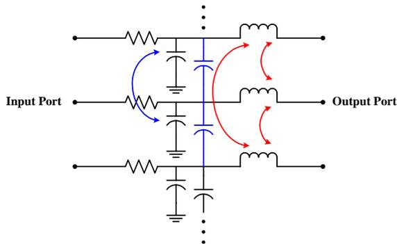
Fig. 3: General lumped model of a package with N interconnections
