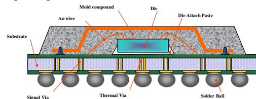
Fig. 1: Cross-section of general 2-layer HS-PBGA
