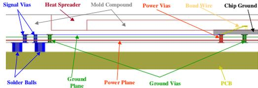
a. Cross-section of the target nets
