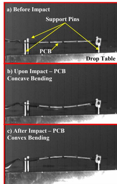
Fig 6. High Speed Digital Images of PCB Bending for Horizontal Orientation Drop.
