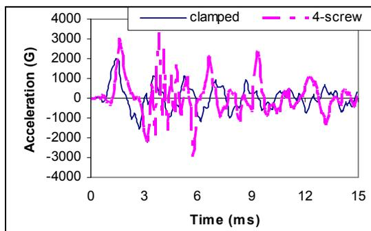
Fig 14. Output Acceleration of the PCB Center for Different Support Conditions.
