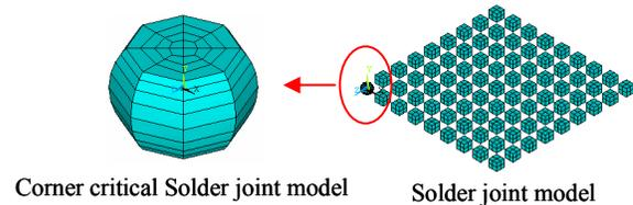
Fig 12b. Fine and Coarse Meshing for Corner and Rest of the Solder Joint Array.
