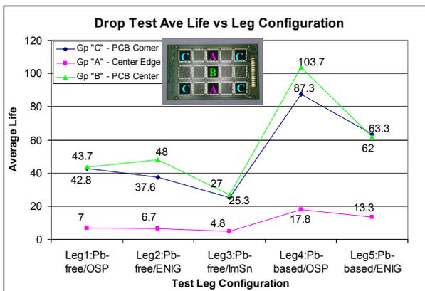
Fig 7. Drop Test Failure Cycles for Different Test Legs.
