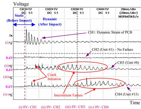
Fig 5. Typical Dynamic Responses for Drop Test - Leg 5 (Pb-based on ENIG) at 78<sup>th</sup> Drop.
