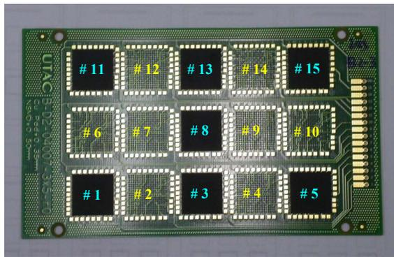
Fig 2. 77x132mm PCB with 15x15mm FBGA Packages.
