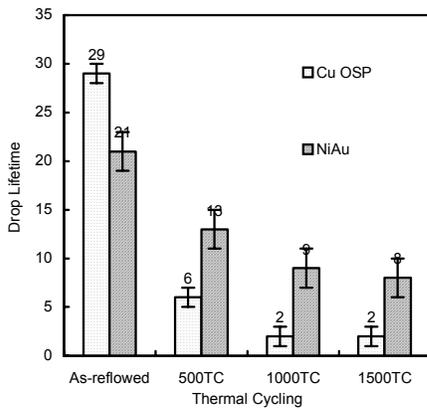
Fig. 11. Drop Lifetime for Units #3 and #13 Before and After Thermal Cycling Aging.
