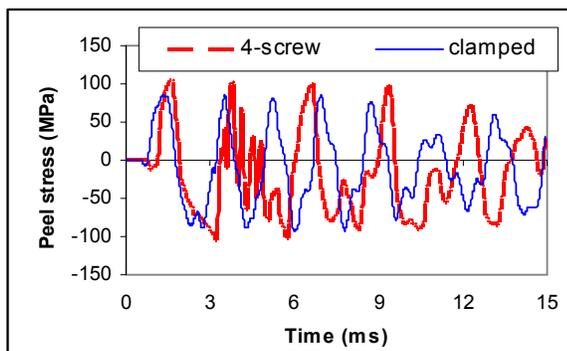
Fig 15. Peel Stress of Critical Node for Different Support Conditions.
