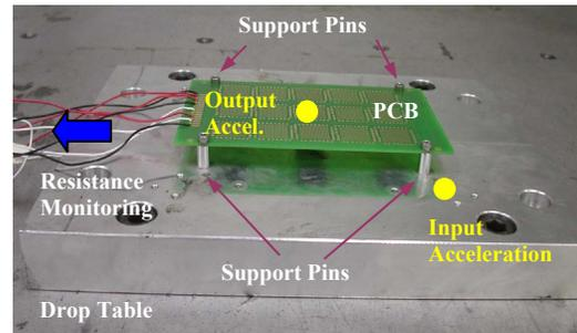
Fig 3. Drop Test Fixture with PCB Mounted onto it.
