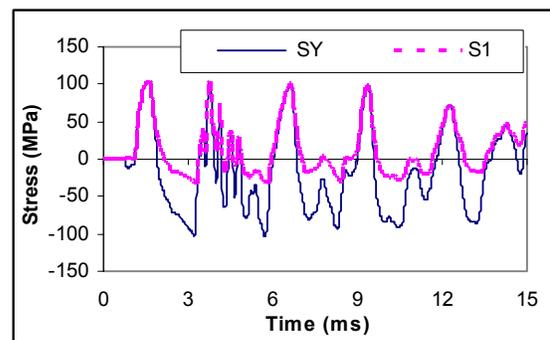
Fig 13. Peel (SY) and First Principal (S1) Stresses of Critical Node for 4-screw Support Condition.
