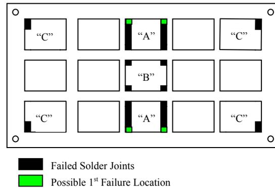
Fig 8. Solder Joints Failure Distribution Across the PCB.
