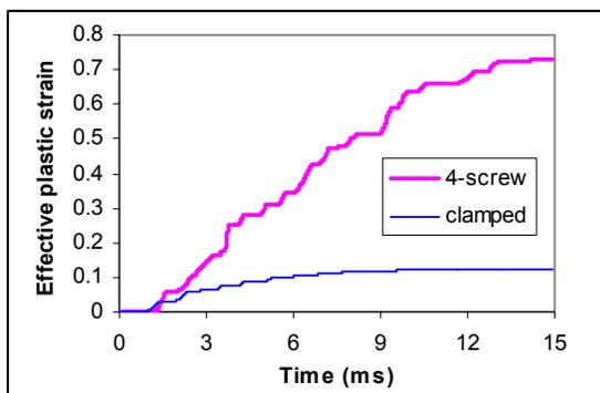
Fig 16. Effective Plastic Strain of Critical Solder Node for Different Support Conditions.
