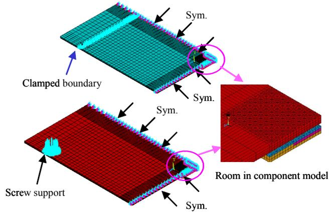
Fig 12a. 3D Quarter FE Model and Boundary Conditions for the FBGA Specimen.
