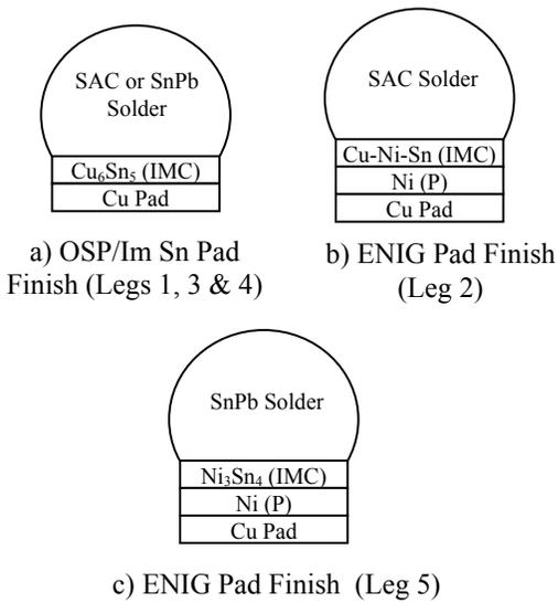
Fig 9. Intermetallic Compound Layers Formation for Legs 1-5.
