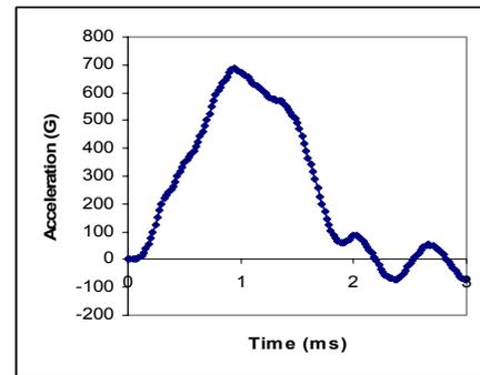
Fig 4. Input Acceleration at the Drop Table Upon Impact.
