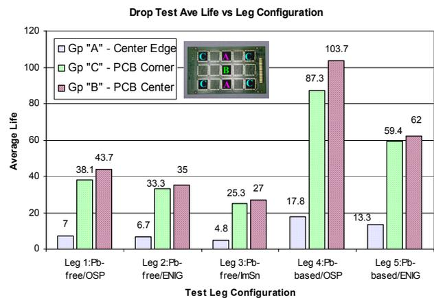
Fig. 3 Drop test failure cycles for different test legs.
