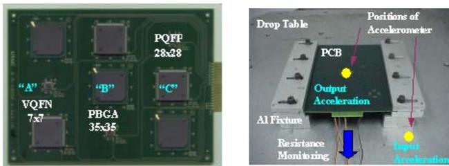
a) PBGA, PQFP and VQFN specimens and clamped boundary
