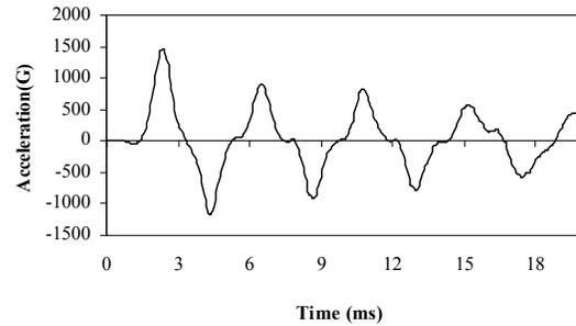
Fig. 2 Output accelerations of PCB center for specimen a.
