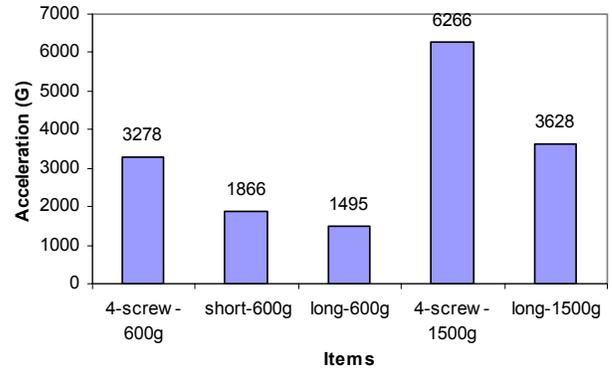
Fig. 16 Peak acceleration of PCB center.
