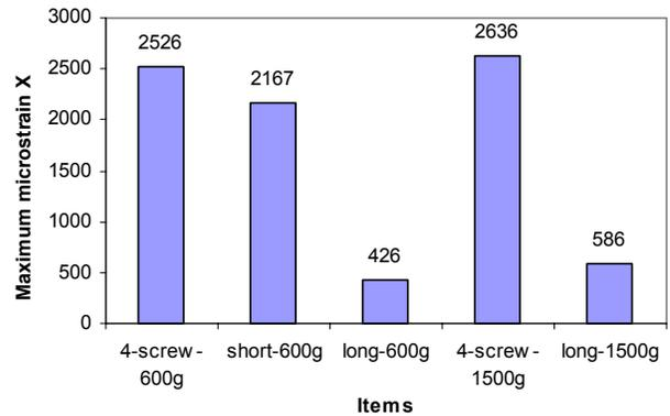
Fig. 17 Maximum PCB longitudinal strain.
