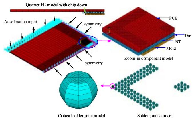
Fig. 6 Quarter FE model for PBGA assembly.
