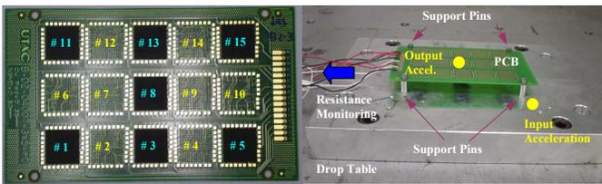
b) FBGA specimen and 4-screw support boundary
