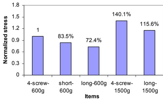
Fig. 19 Boundary and input-G effect on peak peel stress.
