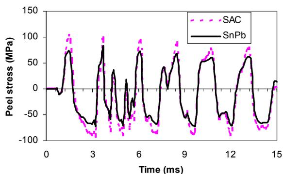
Fig. 22 Peel stress history of critical node for different solder materials.
