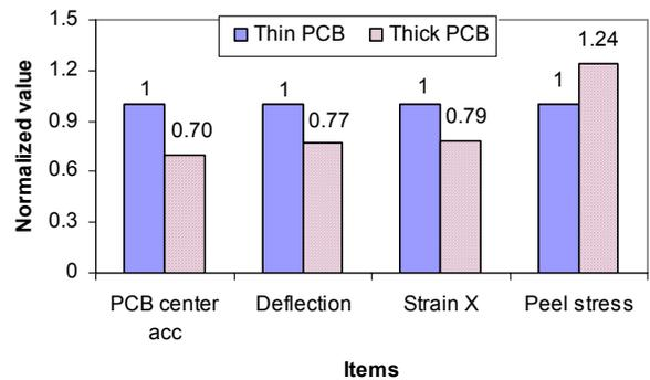
Fig. 21 PCB thickness effect on dynamic response.
