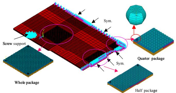
Fig. 9 3D Quarter FE Model for the FBGA Specimen.
