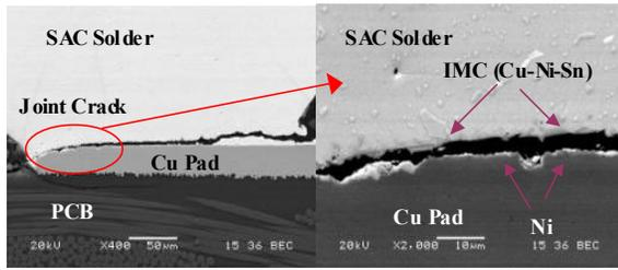
a) Pb-free solder joint failure
