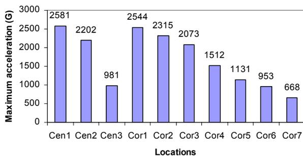
Fig. 11 Maximum acceleration of different PCB locations.
