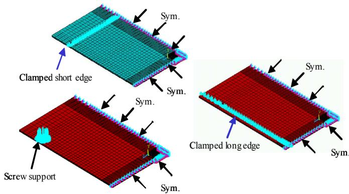
Fig. 14 Three different support boundary models.
