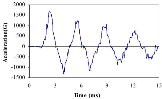
Fig. 7 Acceleration of PCB center from FEA simulation.
