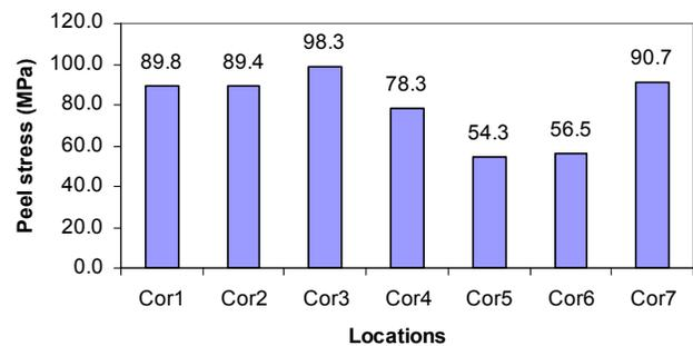
Fig. 13. Maximum peel stress at different solder locations.
