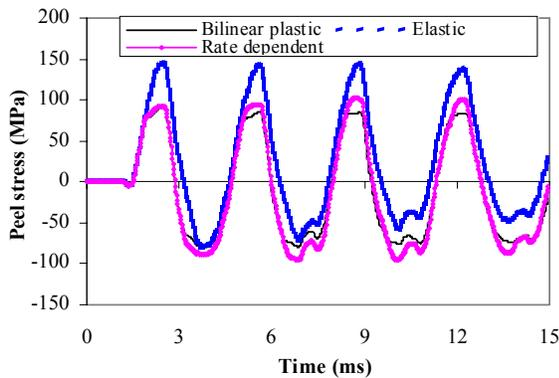
Fig. 8 Peel stress comparison for different solder models.
