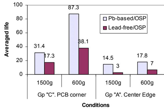
Fig. 5 Drop life comparison for different input-G levels.
