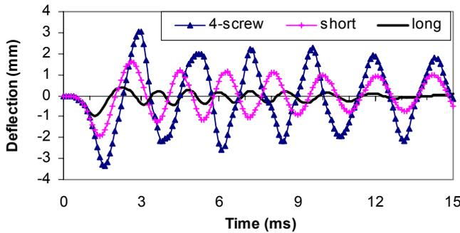
Fig. 15 Deflection history of PCB center for different boundary conditions.
