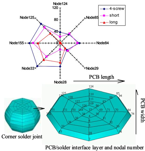
Fig. 18 Nodal peel stress of solder/PCB interface perimeter.
