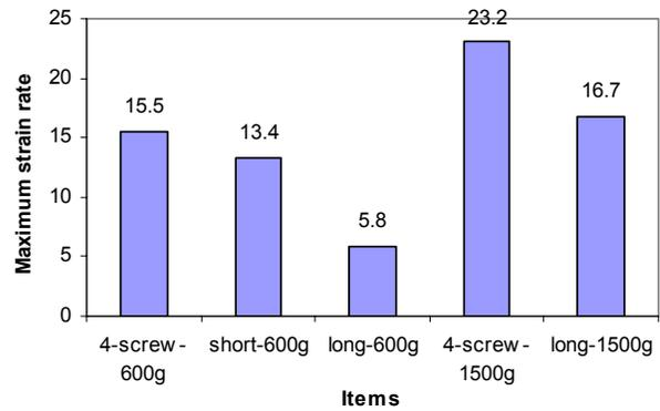
Fig. 20 Peel strain rate of critical interface location.
