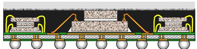
Fig. 4 Package structure (XP-PBGA 40x40mm MCP)
