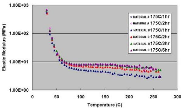
Figure 3: Effect of Temperature on Elastic Modulus For Material A and Material B
