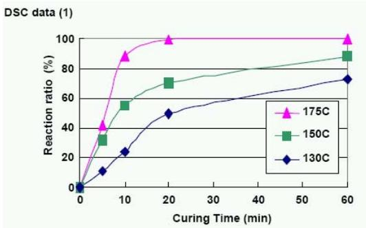
Figure 1: Effect of Curing Time on Reaction Ratio For Material A
