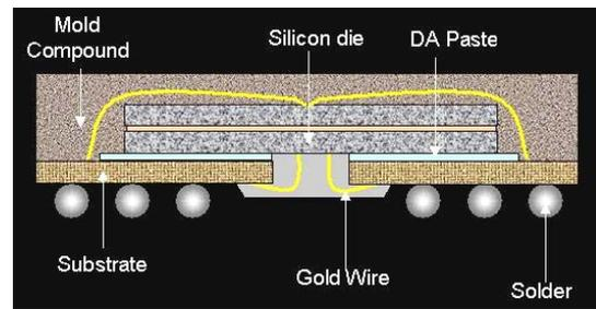
Figure 4: Package Structure of D2-wCSP
