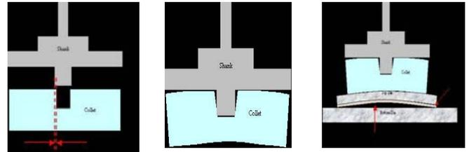
Figure 6: Illustration of Die Warpage Using High Temperature Collet
