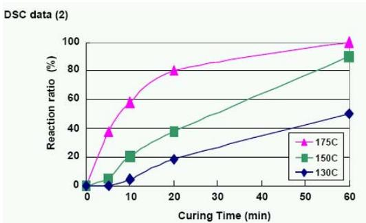
Figure 2: Effect of Curing Time on Reaction Ratio For Material B
