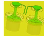
Fig. 3 Differential via together with solder ball studied here.
