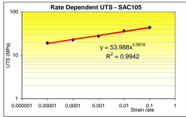
Fig. 11 Relationship between UTS and strain rates of SAC105 at 25°C
