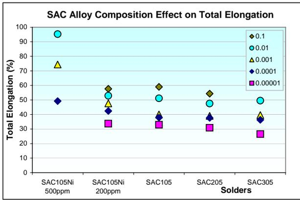
Fig. 15 SAC Alloy Composition Effect on Total Elongation at all strain rates at room temperature
