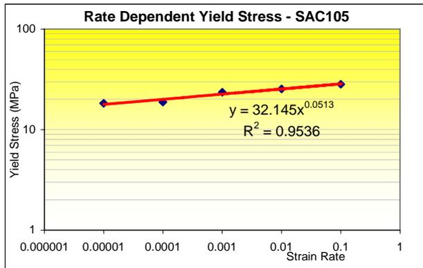
Fig. 10 Relationship between yield stress and strain rates of SAC105 at 25°C
