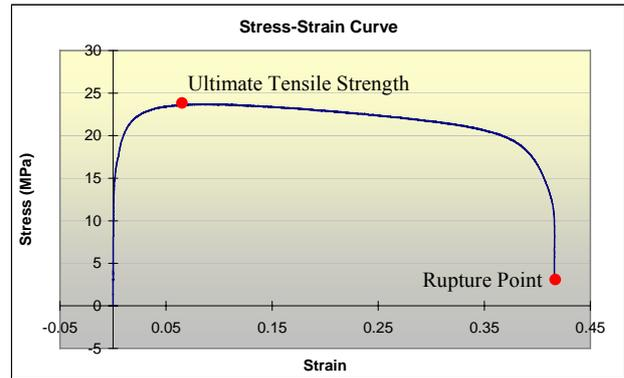
Fig. 4 Stress-strain behaviour for SAC105 under strain rate 0.01 at 75°C
