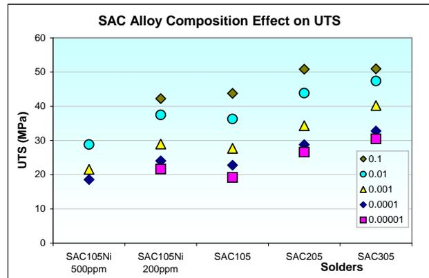
Fig. 14 SAC Alloy Composition Effect on UTS at all strain rates at room temperature
