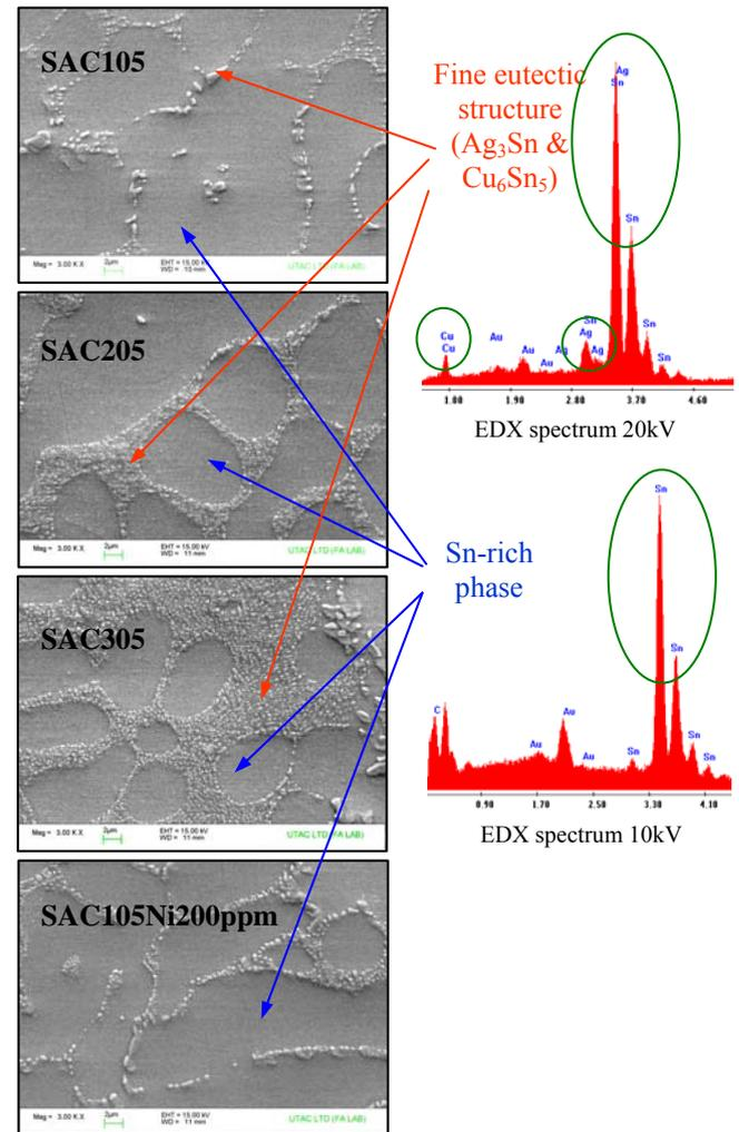
Fig. 19 SAC bulk solder microstructures
