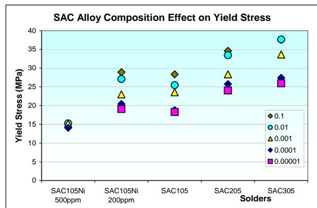
Fig. 13 SAC Alloy Composition Effect on Yield Stress at all strain rates at room temperature
