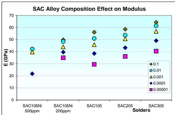
Fig. 12 SAC Alloy Composition Effect on Modulus at all strain rates at room temperature
