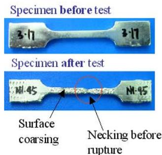
Fig. 3 Typical solder failure mode
