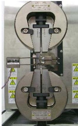
Fig. 2 Test setup with extensometer affixed
