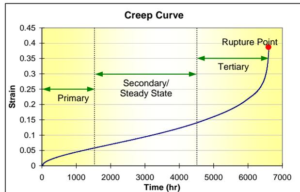
Fig. 5 Creep curve for SAC105Ni0.02 undergone isostress 20MPa at 25°C
