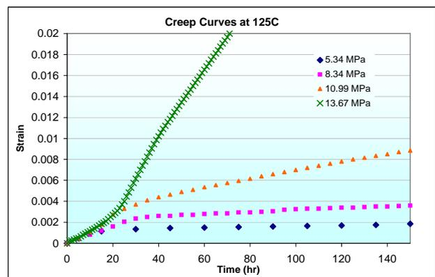
Fig. 17 Creep curves of SAC105Ni200ppm at isostress levels at 125°C (until 150 hours)
