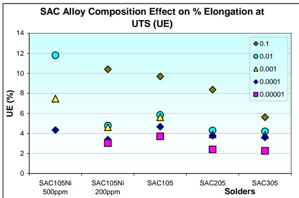
Fig. 16 SAC Alloy Composition Effect on % Elongation at UTS at all strain rates at room temperature
