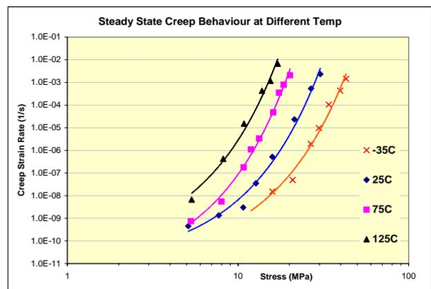
Fig. 18 Steady state creep rate of SAC105Ni200ppm at different temperatures
