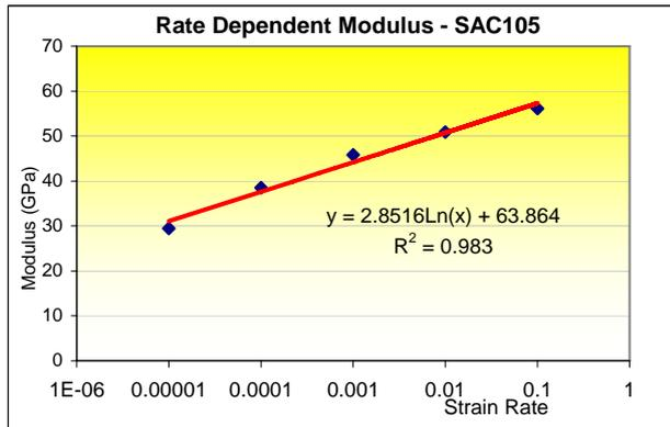
Fig. 9 Relationship between modulus and strain rates of SAC105 at 25°C
