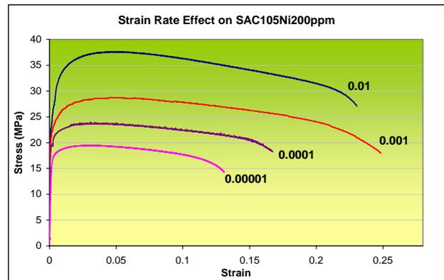
Fig. 7 Stress-strain curves of SAC105Ni200ppm at different strain rates at  $25^{\circ}\text{C}$
