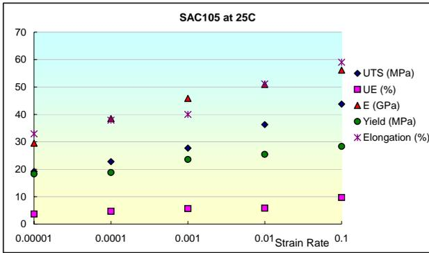
Fig. 8 Effects of strain rates on material properties of SAC105Ni200ppm at 25°C
