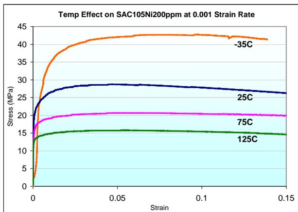
Fig. 6 Stress-strain behaviour of SAC105Ni200ppm at  $0.001\text{s}^{-1}$  at different temperatures
