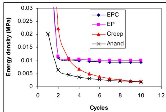
Fig. 13 Energy density accumulation per cycle for bending simulation with 1.5mm deflection and 125°C.
