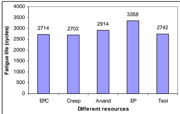
Fig. 6 Fatigue life based on different constitutive models.
