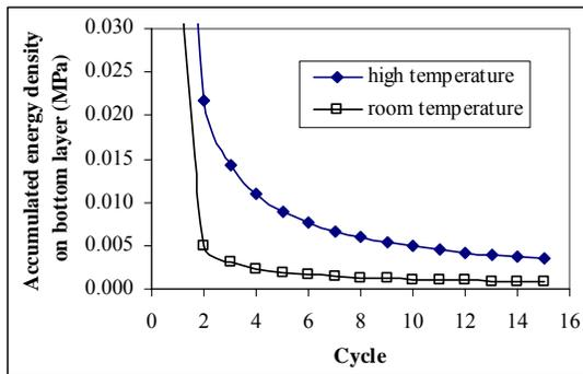
Fig. 10 Energy density accumulation per cycle for bending simulation with 2.16mm deflection and Anand model.
