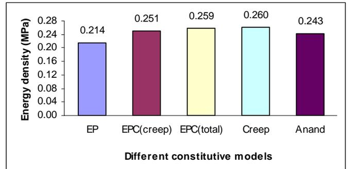
Fig. 4 Strain energy density accumulation per cycle for different constitutive models.
