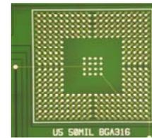
Fig. 1 PBGA layout and solder distribution pattern.
