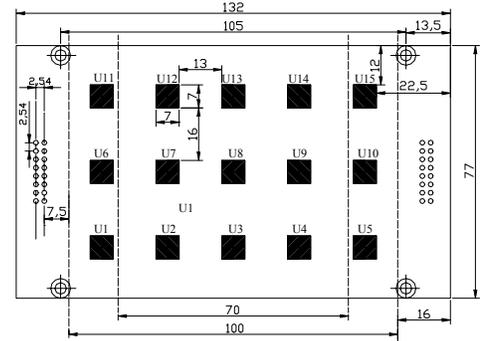
Fig. 7 Layout of VQFN specimen.
