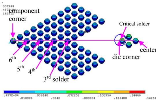
Fig. 3 Plastic work density distribution on solder joint.
