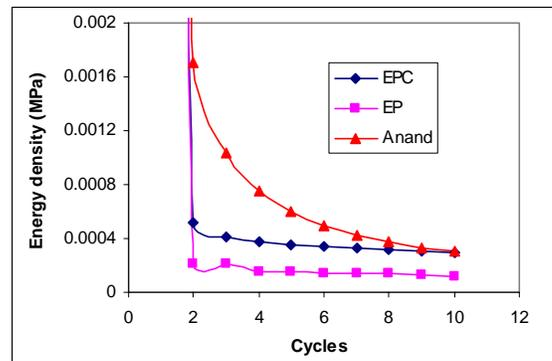
Fig. 12 Energy density accumulation per cycle for bending simulation with 1.5mm deflection and 25°C.
