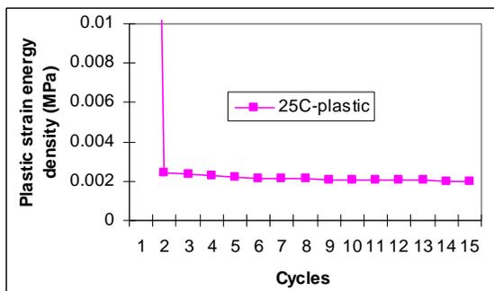
Fig. 11 Energy density for bending simulation at 25°C with 2.16mm deflection and EPC model.
