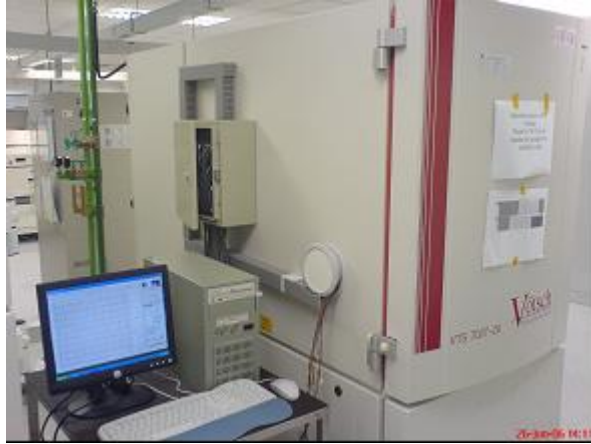
Figure 3: UTAC in-house TC chamber with in-situ monitoring system
