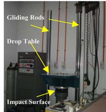
Fig. 2. Lansmont model 65/81 drop impact tester.
