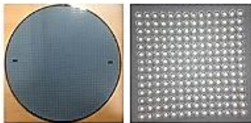
Figure 6. Molded full wafer and die BGAs side mold compound support view
