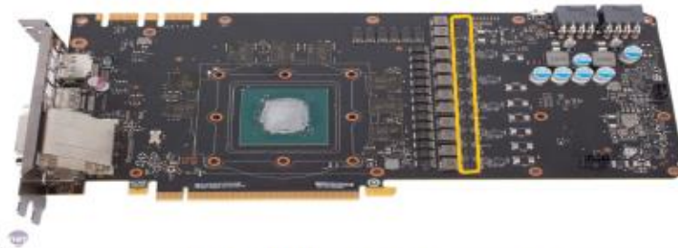
Figure 4a. GIGABYTE-GeForce-GTX-1080 VGA Card with Discrete MOSFET and driver IC.
