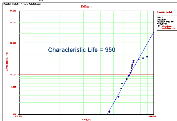
Figure 17: Weibull plot for drop test characteristic life
