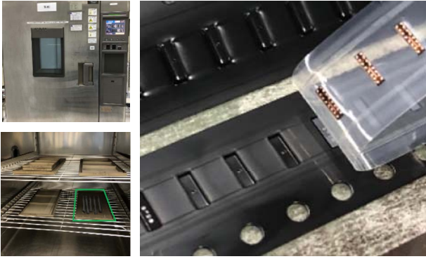
Fig. 1. Example of DOE setup and samples showing the simulation of die sticking to cover tape failure.
