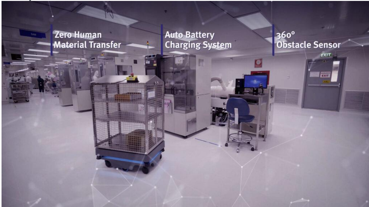
Automated Guided Vehicle – Courtesy of UTAC, 2021
